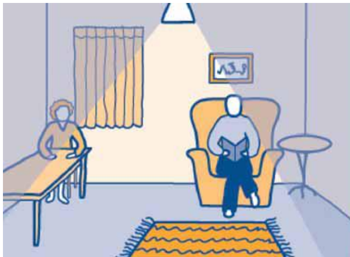
Figure 1: Illustration showing the narrow area that is lit when one central ceiling light with a lamp shade is used to light a room. Two people are in the room, one sitting at a table on the left and the other reading in an armchair on the right. A triangle of light is cast in the room from the central light fitting, with only half of the table being fully lit.
